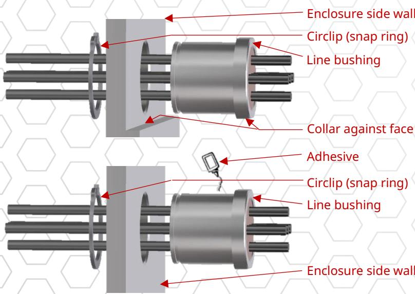
Fixing details for installation with Circlip DIN 472 (for hole):
