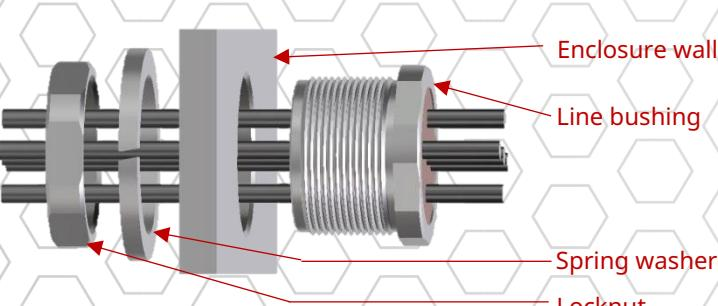
Also applicable for threaded blind plug / blanking plug and twin-path version.
