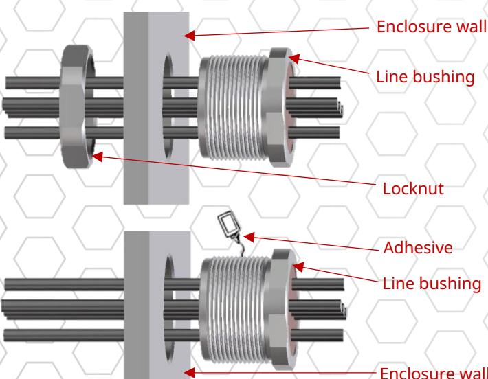
Fixing details for application with vibrations:
